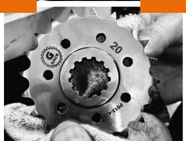
Gandini front sprockets are made at the same as the rear from solid forged extruded bares, made in 18NICRMO5 steel, finished with hardened and tempered heat treatment.
