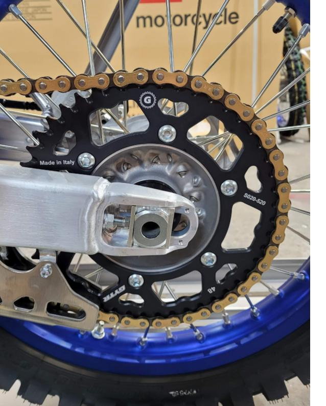
Gandini rear sprockets are made from solid, from forged extruded bares, in special hard anodized aluminum 7075-T6 alloy.
